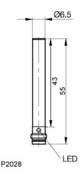
Inductive Sensors BES 516-3025-G-E5-C-S49 D6.5 x 55 normally-closed Sn=2mm shielded
